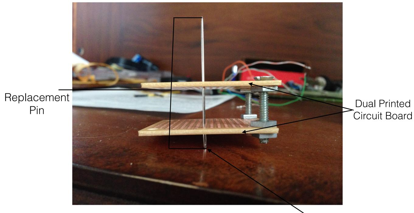
Hole in "pin" in which memory wire will be put through
