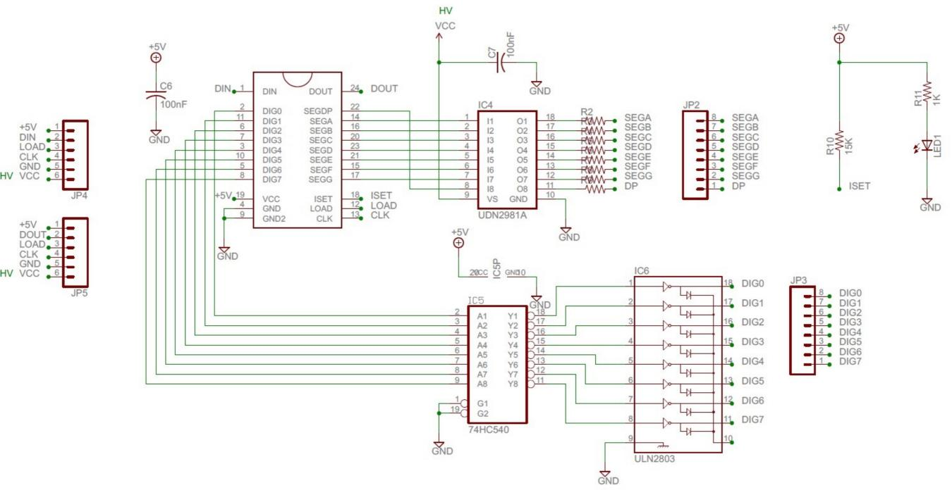
These are schematics that allow the setup of MAX7219 with high power. The chip alone cannot output high currents but with another chip, UDN2981A, a 8-channel source driver it can output high current to the pins.
