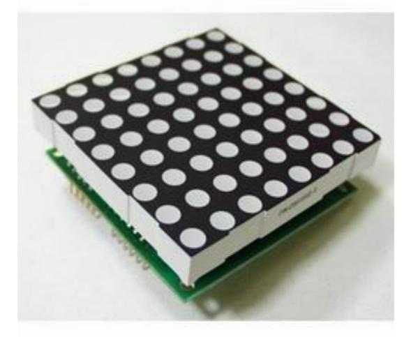
Using a similar design, I could remove the LEDs from this LED array and connect the wire from the reading pins for my Braille project. This would simplify installation and be much neater. The chip used to control the LED array, MAX7219, can control the 8x8 LEDs but it cannot work directly with the Braille display because the maximum current is too low.
