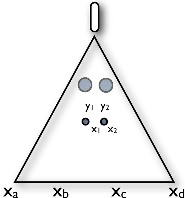
Figure 5 shows how the wiimote “sees” the infrared LEDs. The farther away, the smaller the LEDs; the closer, the bigger the LEDs.
