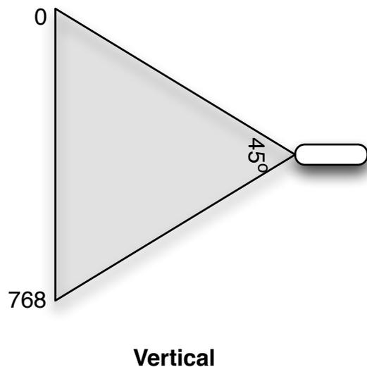
Figure 4 shows an important factor of this project; the range of the wiimote. The range of the wiimote (at a 45° angle) horizontally is 1024 pixels and vertically it is 768 pixels
